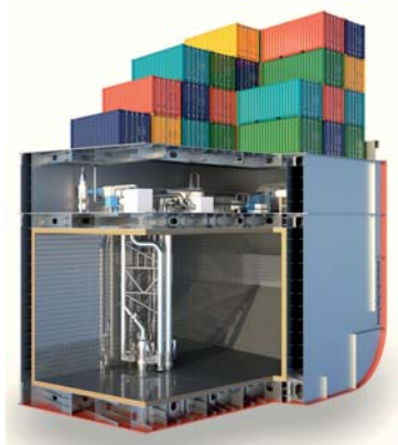
Example of a large coastal container ship converted through "jumboisation" and insertion of a vessel section containing the LNG fuel tank and the gas preparation unit.
